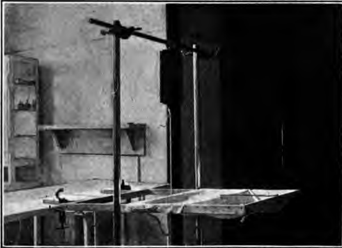
Apparatus showing method by which the strength of the grasping reflex is measured. The baby is laid in the canvas crib. The weight of the baby immediately registers. The rod is then put in the baby's hand and raised. The decrease in the weight registered shows the strength of the pull.
